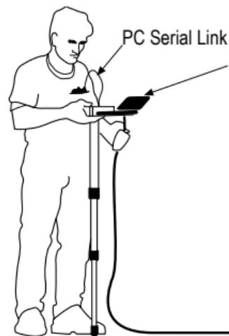
Compact PC mounted to Unipod in left hand or in pocket with display visible to operator
